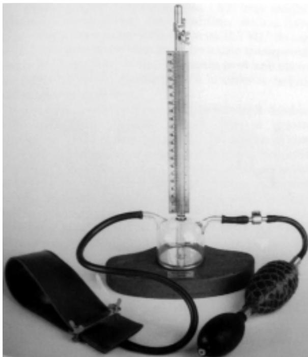
**Figure 2.** The Riva-Rocci sphygmomanometer. Reprinted with permission from Brown WC, O'Brien ET, Semple PF. The sphygmomanometer of Riva-Rocci 1896–1996. *J Hum Hypertens* 1996;10:723–4.
