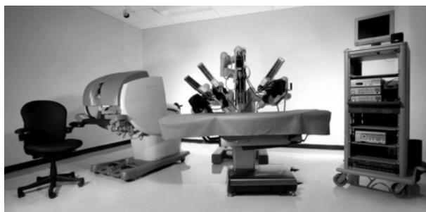
**Figure 1.** Robotic cart with 4 arms. (Reproduced with permission from Intuitive Surgical, Inc. Copyright © 2005.)
